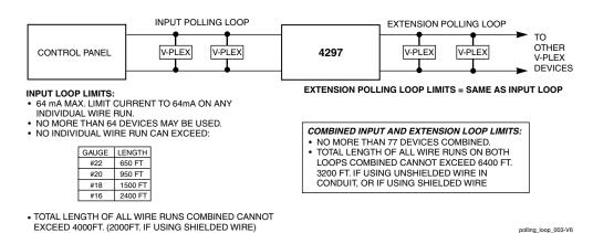
Figure 3-14: Polling Loop Connections Using One 4297 Extender Module
