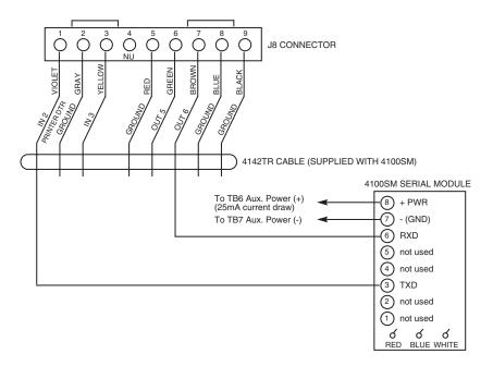
Figure 7-1: Direct-Wire Downloading Connections
