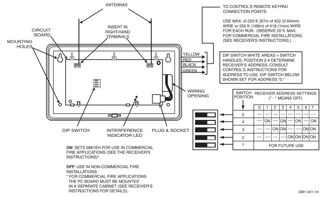
Figure 3-16: RF Receiver (cover removed)
