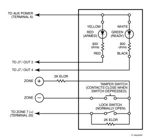
Figure 3-18: Remote Keyswitch Wiring
