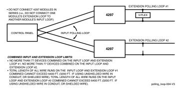
Figure 3-15: Polling Loop Connections Using Multiple Extender Modules NOTE: The input loop limits stated in Figure 3-14 apply to Figure 3-15 as well.
