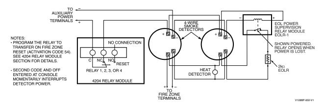
Figure 3-11: 4-Wire Smoke Detectors
