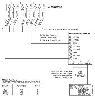
Figure 3-20: 4100SM Using a Serial Printer
