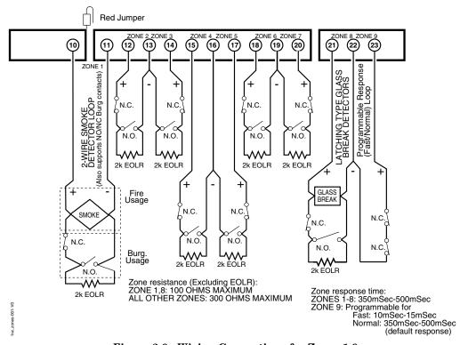
Figure 3-9: Wiring Connections for Zones 1-9
