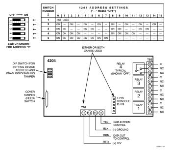
Figure 3-17: 4204 Relay Module
