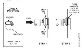
Figure 3-1: Installing the Lock
