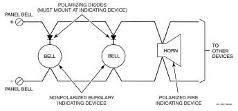
Figure 3-7: Wiring Nonpolarized Burglary Devices
