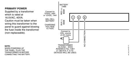
Figure 3-23: 1361 Transformer and Battery Connections
