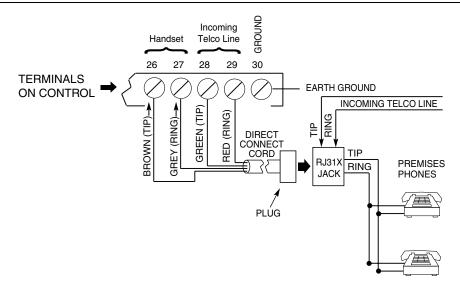
Figure 3-8: Telephone Line Connections
