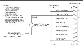
Figure 3-19: Remote Keypad Sounder Wiring
