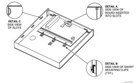
Figure 3-3: Mounting the PC Board
