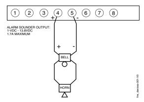
Figure 3-6: Wiring Polarized Fire Devices
