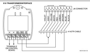
Figure 3-24: 1361X10 Transformer Connections
