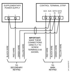
Figure 3-5: Using a Supplementary Power Supply
