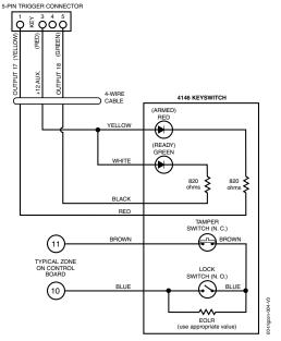
Figure 10. Keyswitch Wiring Connections
