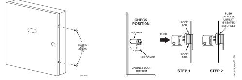
Figure 1. Installing the Door and Cabinet Lock
