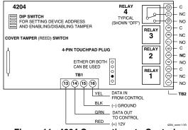
Figure 11. 4204 Connections to Control
