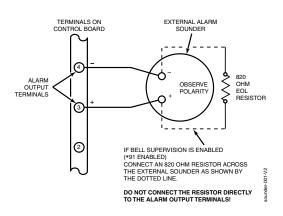
Figure 5. Sounder Wiring (Supervised)
