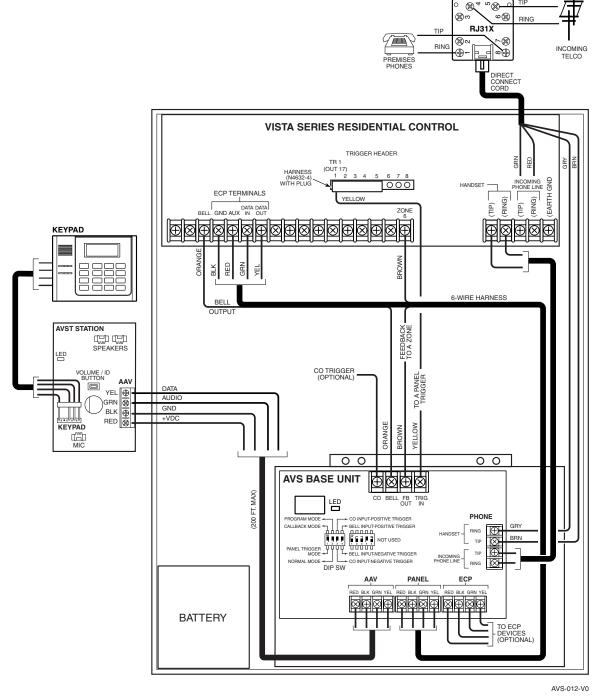
Figure 16. Connection of AVS Module
