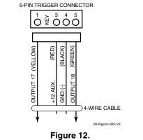
On-Board Trigger Connector with 4-Wire Cable
