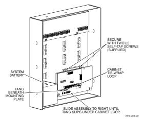
**BATTERY NOTE:** When using a 7AH battery, mount the battery vertically on the bottom left-hand side of the cabinet, with the terminals facing down and right (negative terminal closest to the PC board bracket).
