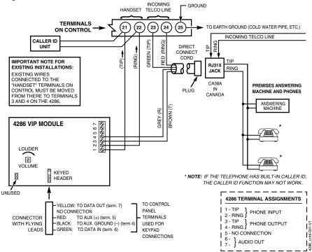
Figure 13. 4286 Phone Module Wiring Connections
