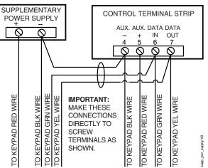
Figure 4. Using a Supplementary Power Supply
