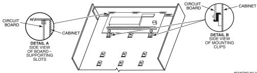
Figure 2. Mounting the PC Board
