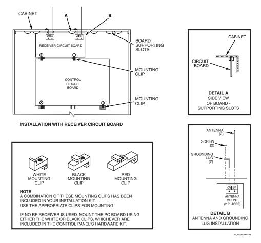
Figure 3. Mounting the PC Board and RF Receiver
