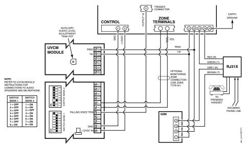
Figure 15. Connection of UVCM Unit When Using a 4286 Phone Module
